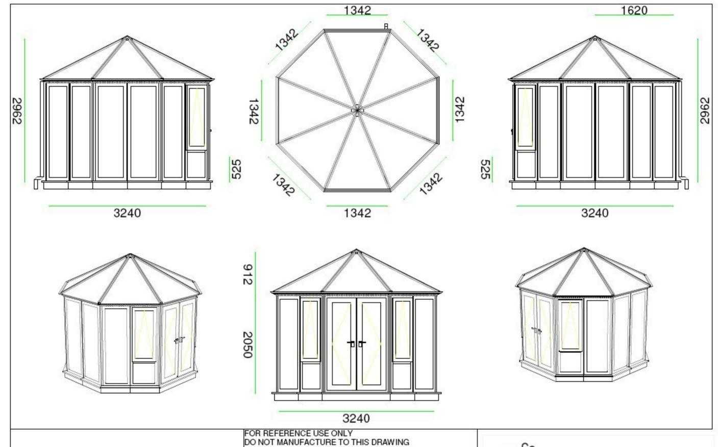
DO NOT MANUFACTURE TO THIS DRAWING ALL ROOF DIMENSIONS ARE APPROXIMATE Frame dimensions shown are internal sizes. Height shown does not include height of cresting. All dimensions are in millimetres. SILLS WILL EXTEND THE WIDTH BY 300MM AND THE PROJECTION BY 150MM.
